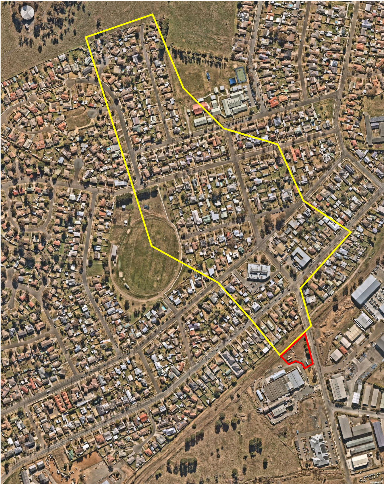
Figure 1. Aerial image of the development site (red) and the contributing catchment area to the north and northwest of approximately 20 hectares (yellow) which generates rainwater and surface water runoff that burdens the site. It is noted that the surface types within the catchment are fairly uniform with low density residential dwellings, roads corridors, and open public spaces. The development site and adjoining lands to the east and south transition into industrial developments.
